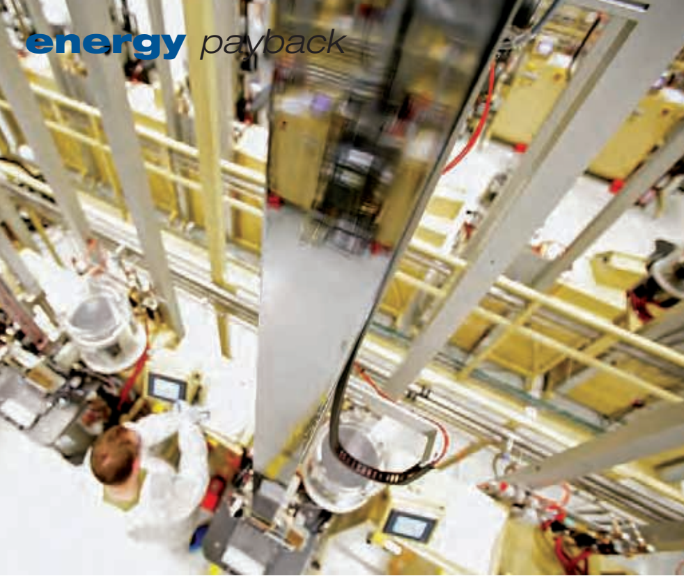
The Evergreen Solar manufacturing process grows string-ribbon crystals at the thickness of the finished cell, saving silicon waste and reducing embodied energy by as much as 25%.
